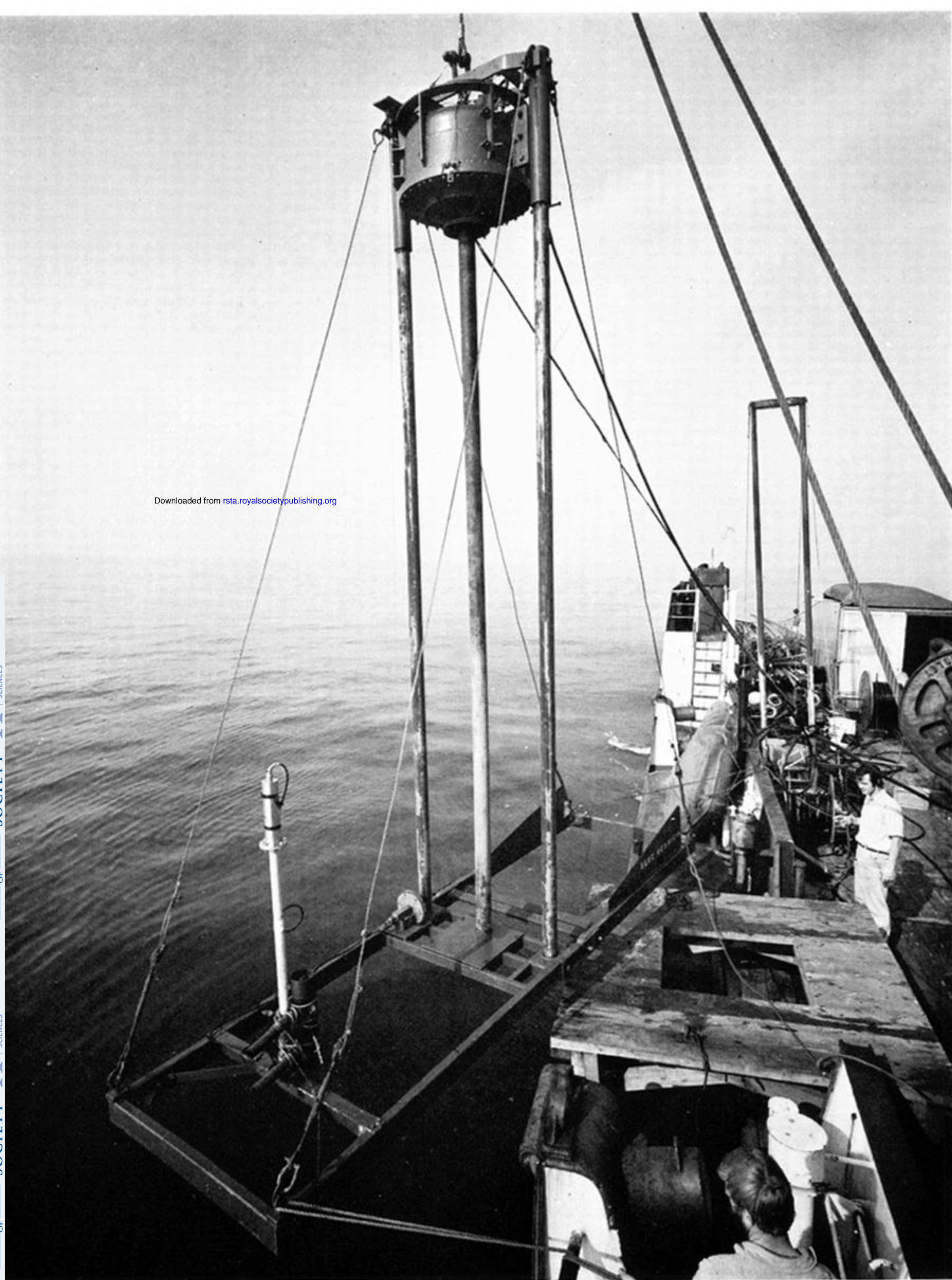
FIGURE 6. IOS (Taunton) vibrocorer used to obtain cores from Start Bay. Photograph by permission of The Netherlands Rijkswaterstaat.
